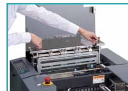
DC-516 Pro comes with one cutting module, one slitting module and one creasing module
