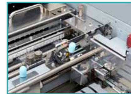
Automatic REG mark scanner compensates for image shifting in the horizontal direction
