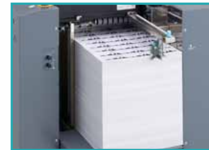
High pile feeder with 8-belt air suction feed system
