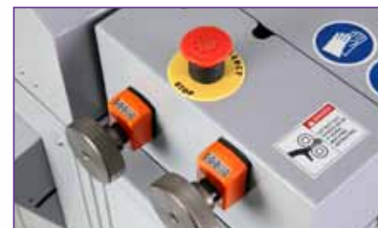
Coating roller gap dials for one-time adjustments
