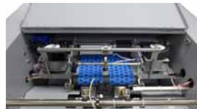
SF-300 Suction Feeder with double feed detection
