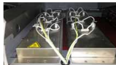
Optional dual IR kit for KMBS and Ricoh prints
