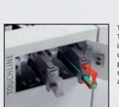
The creasing and perforating tools are automatically detected and the relevant pressure is automatically set. No manual adjustments
