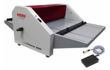
This creasing and perforating machine with a working width of 18" is designed for the final processing of graphic materials up to  $18" \times 23.4"$ . Creasing enables high-quality folds of digitally printed paper. The machine can also be controlled via a foot pedal. The GoCrease<sup>TM</sup> 4000 is built with high quality anvil perforation, as well as 3 different creasing channel widths.
